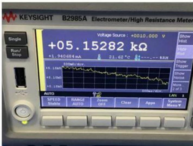
Fig 19 Insulation resistance MLCC failure using the B2987A Electrometer/High Resistance Meter. Note the decay in resistance vs. time.
