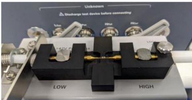
Fig 7 MLCC in 4TP measurement and compensation test fixture
