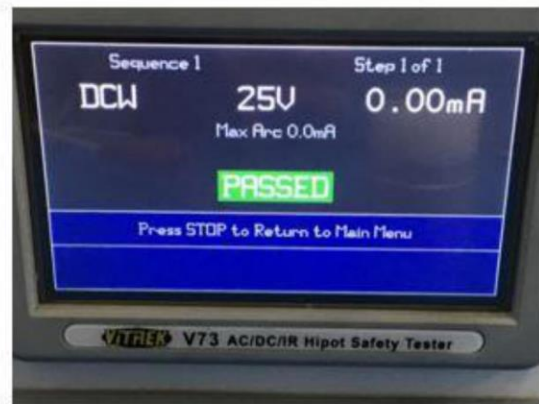
Fig 21 Dielectric Withstanding Voltage Testing using the Vitrek V73 AC/DC/IR hipot Hipot tester showing that the device passed the 2xVoltage rating for the Class II MLCC part no. C2012JB1A476M125AC.
