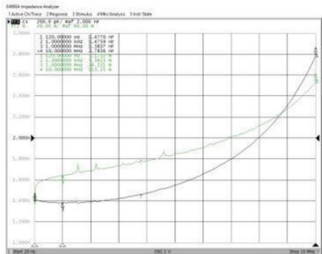
Fig 9 Class-II MLCC capacitance measurement. C0805C152KDRACAUTO Capacitance change vs. Frequency (20Hz to 10 MHz)
