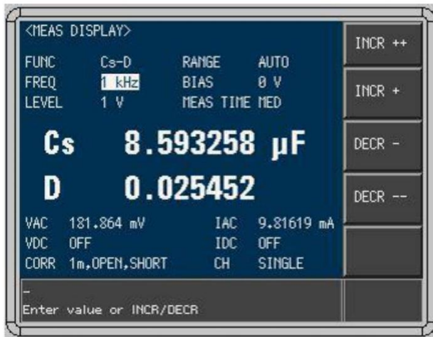
Fig 11 Capacitance measured without ALC. The Testing level set to 1.0V, however the Voltage monitor showing only using 181.864 mV
