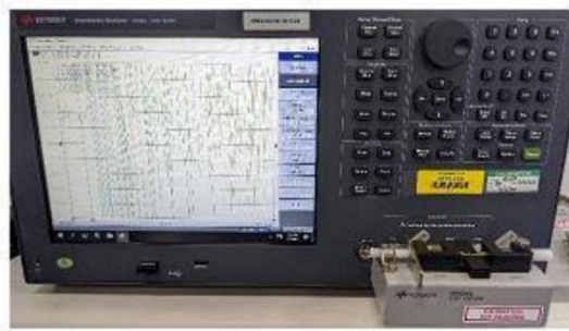
Fig. 5 Photograph of the Keysight E4990A and test fixture 16034G used to make the capacitance test.
